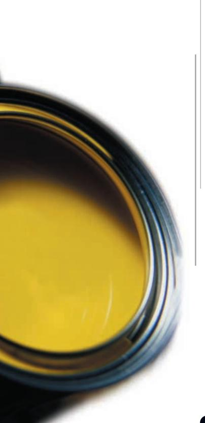
POLYOX Water-Soluble Resins are nonionic, high molecular weight water-soluble poly (ethylene oxide) polymers. Molecular weights range from 100,000 to about 8,000,000. They exhibit many properties that are typical of other classes of water-soluble polymers – lubricity, binding, water retention, thickening, and film formation.
