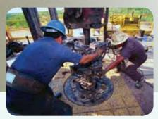
A Molykote<sup>®</sup> anti-seize paste with metal-free solid lubricants reduced thread failure rates on rotary drilling equipment and helped maintain production schedules.
