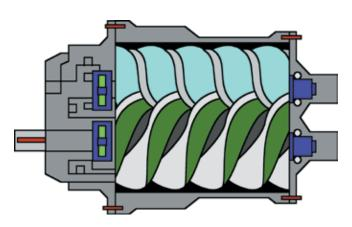
In a compressor, the fluid is recirculated in a closed system, and it flows from the compressor to the separator. From there it is pumped to a cooler, through a filter, and back again to the compressor. Breakdown of the lubricant or its capabilities causes compressor problems.
